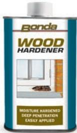
Bonda Wood Hardener is a purpose formulated hardener for rotten and decayed wood. The resin penetrates into the fibres where the moisture hardens the resin. The hardening process is not affected by temperature. The wood fibres are bonded together providing a consolidated structure and a tough hard surface, sealing the surface from further moisture penetration.
