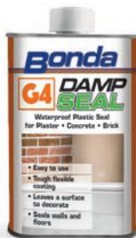
A moisture curing single part polyurethane varnish ideal for sealing damp porous surfaces prior to using release agent. Used as damp proof floor sealing, pond sealing, sealing concrete prior to GRP sheathing where alkali in concrete can react with resins. Also an ideal coating for plug surfacing before taking mould as release agents and resins do not attack G4.
